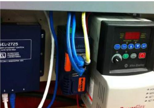
The eWON Cosy 131 router offers easy remote access to McMaster PLC laboratory
