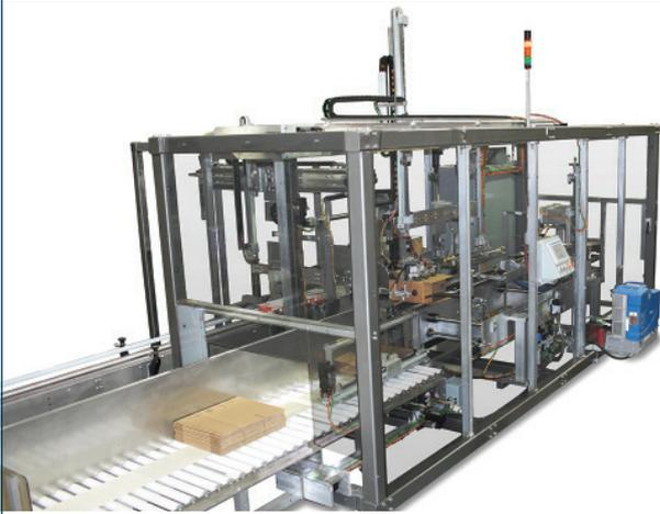
The TR-QCP Transrector Robotic Case Packer features a case transporting system never before seen in the case packing industry.
