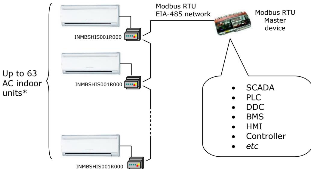
\* Up to 63 Intesis devices can be installed in the same Modbus RTU bus. However, depending on the configured speed, the installation of Modbus Repeaters may be required
