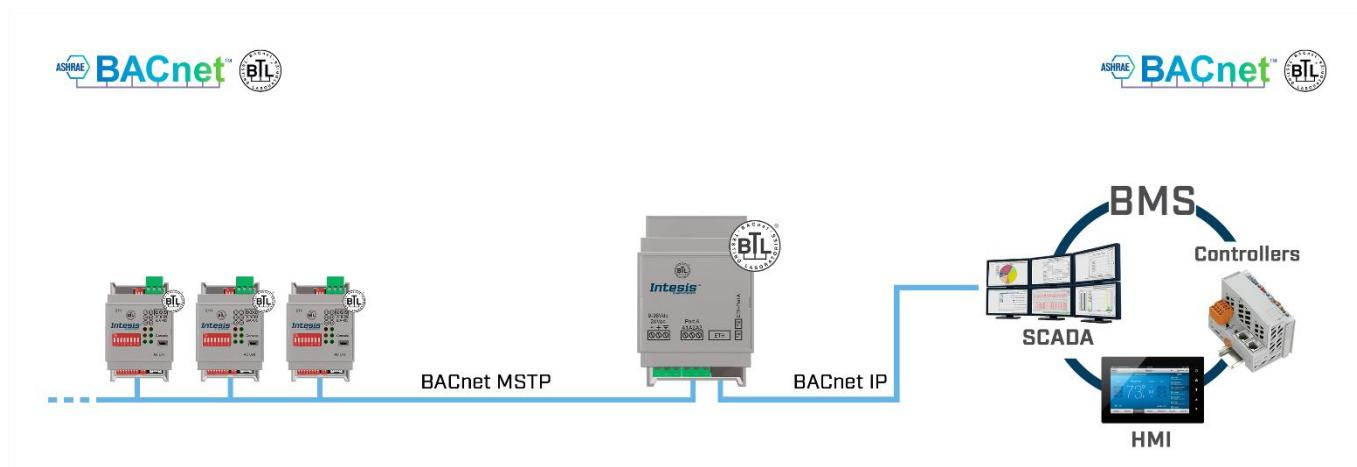
Routing between BACnet MS/TP and BACnet IP networks
