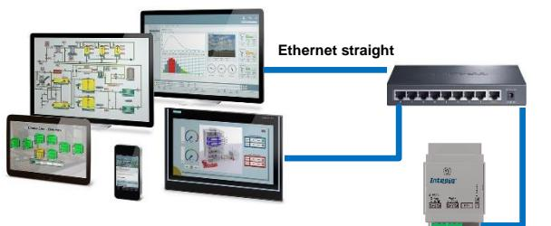
BACnet IP connection using switch/hub and straight cable
