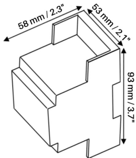
**IMPORTANT!** Leave enough clear space to wire the gateway easily and for the subsequent manipulation of elements.
