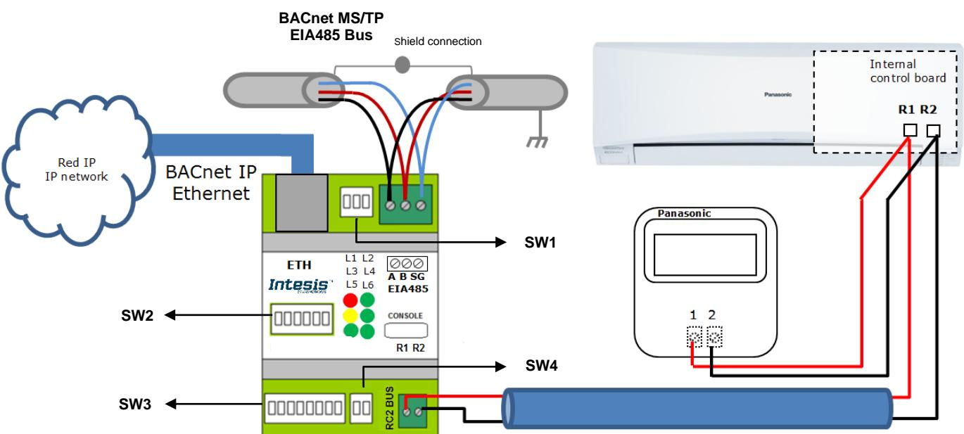
Figure 2.2 Connection diagram
